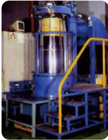
■ Automation Winding Machine for High Voltage Coils
